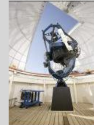
32" Ritchey-Chrétien Telescope Tarleton State University
