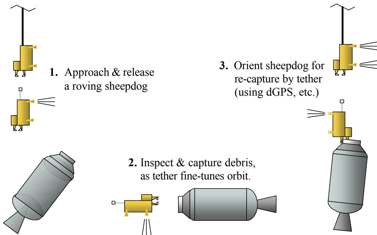
Figure 7. Two-stage Cooperative “Two-Dog” Capture of Passive Objects by Tether
