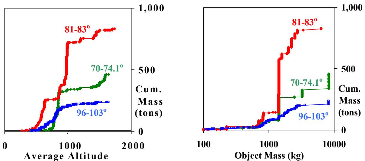
Figure 3. Key characteristics of the 3 largest inclination clusters of debris in low earth orbit.
