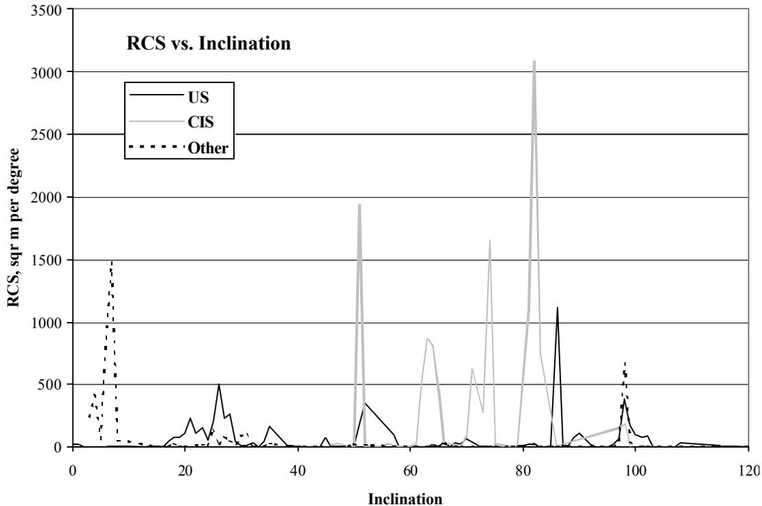
Figure 1. Total Radar Cross-section (m<sup>2</sup>) vs Inclination for Objects in Low Earth Orbit
