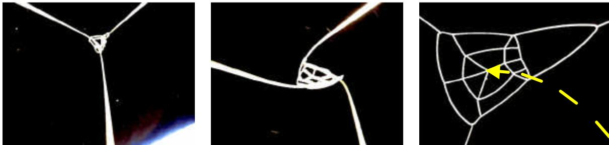
Figure 6. Net spin-up viewed from support, with desired payload trajectory shown in frame 3.
