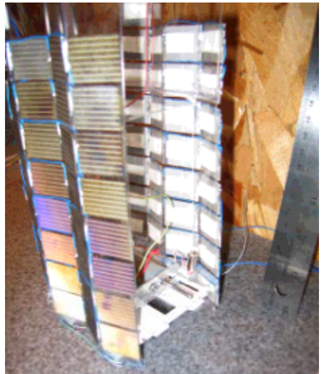
Figure 3: Climber built by Jack Buffington that won the 2004 ribbon climbing competition of the Robotics Society of America. The climber is shown with its photovoltaic arrays folded up. During ascent the arrays fold down.
