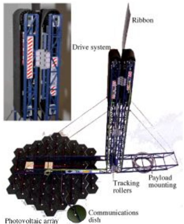
Figure 2: Model of a complete climber system. The inset shows the details of the drive system.
