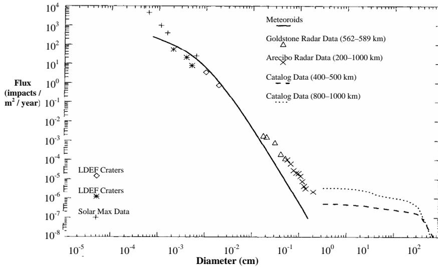
**Figure 2, Impact Rates for Meteoroids and Orbital Debris<sup>2</sup>**
