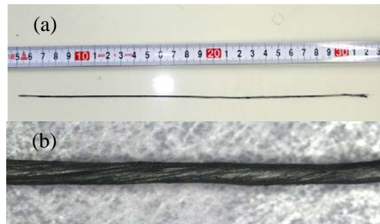
Fig. 6: (a) A 27cm-long CNT spun fiber. (b) Magnified view of the fiber.
