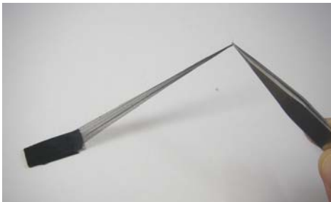
Fig. 4: CNT web is drawn by tweezers from CNT array.
