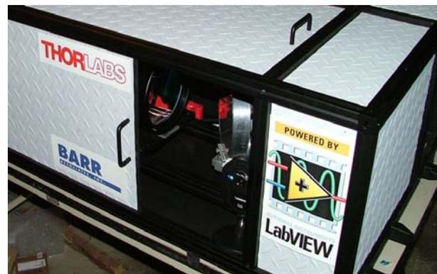
Fig. 1: KCSP Tracking Box with exit lens, tracking mirror, and sheeting air tips.
