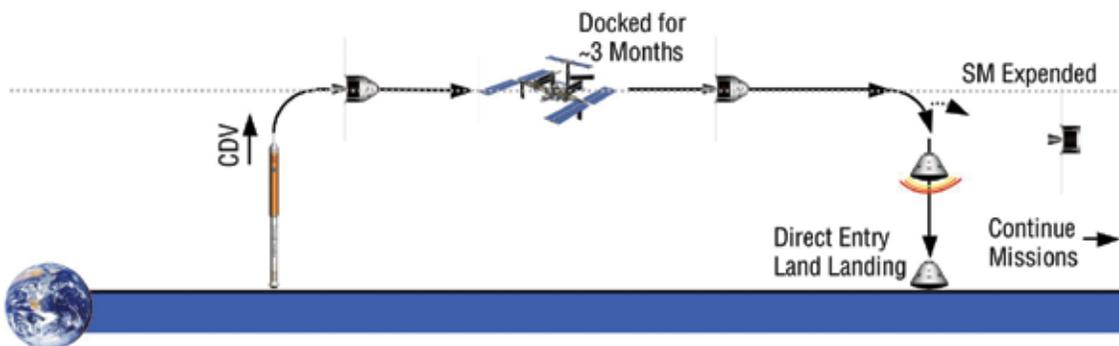
Figure 2-4. Pressurized Cargo Transport to and from ISS DRM
