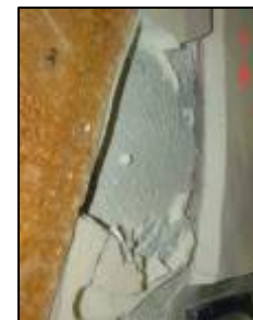
Delamination observed under LH2 IFR
