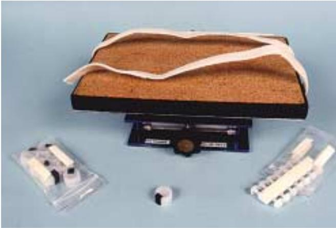
**Figure 3.** This worktable allowed for a variety of procedures to be performed in the GPWS. The table was covered with an absorbent pad, and equipment could be attached to the table either with pins into the cork or by Velcro straps that attached to the Velcro on the sides and bottom of the table. Height was adjustable.
