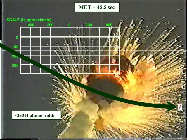
~1700+ ft-dia debris cloud grows off the frame in ~ 3 seconds – w/ no fragments giving indication of slowing (i.e. no fragment has begun to visibly arc with gravity, yet)
