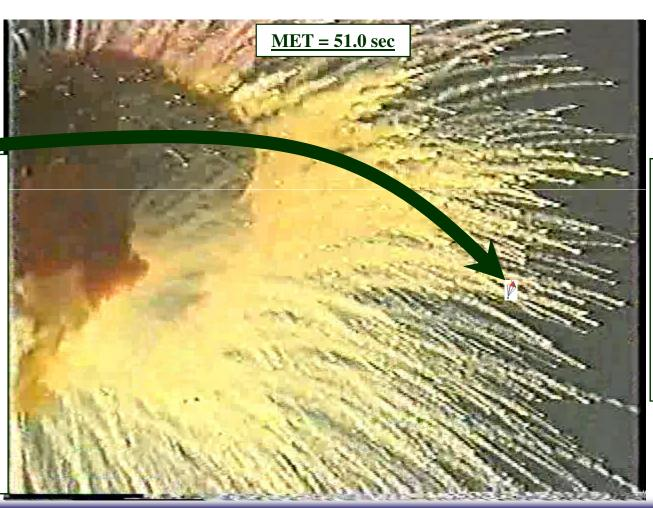
Debris cloud continues growing at ~200 fps, ~9 seconds after destruct, – w/ moderate signs of fragments slowing (i.e. fragments have slightly arced with gravity)
