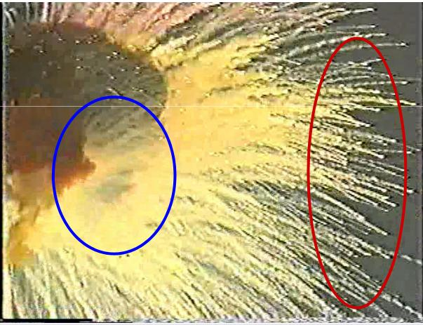
A dense "shell" of fragments, expanding as a hollow sphere
