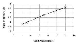
Fig. 3: Relation of phase orbit period and eclipse time
