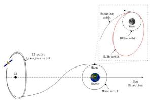
Fig. 4: Flight profile of CE-2 Lagrange L2 Point Mission
